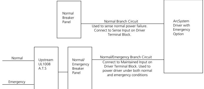
If normal power to the sense input is lost, the driver will force the luminaire on at 100% overriding all other control signals. There is no control of the driver/luminaire via DMX until normal power is restored at the sense input.
